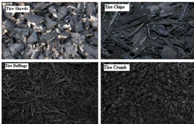
Fig. 1: Typical shapes of different processed used Tires [29].
